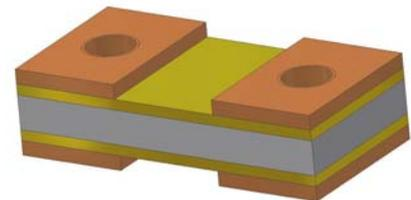
Figure 3. PVS Construction for 0603, 0402, 0201 Surface Mount Device
