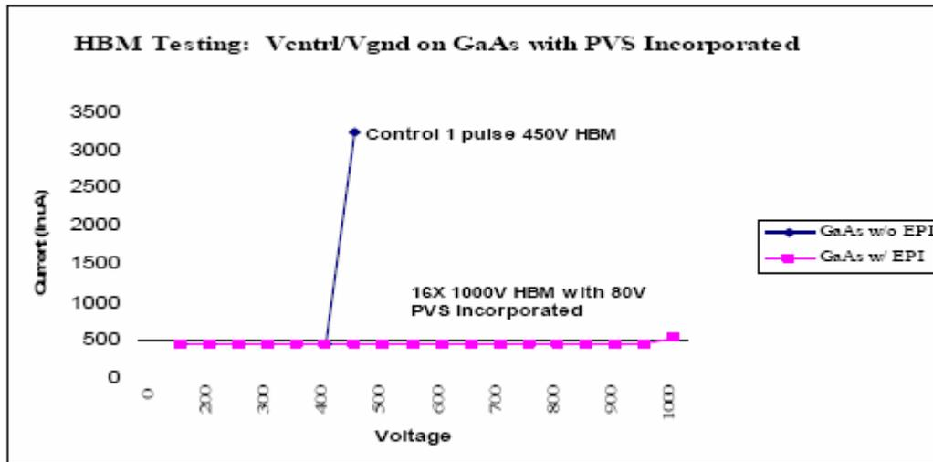
Figure 4: HBM ESD survivability of GaAs IC increases from 450 to 1000 V with 80V trigger EPI-FLO™ surface mount device.
