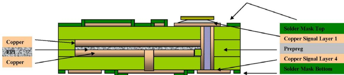
Figure 1 Fabrication Design for embedded EPI-CORE™ ESD protection layer in a 4 layer RF module.
