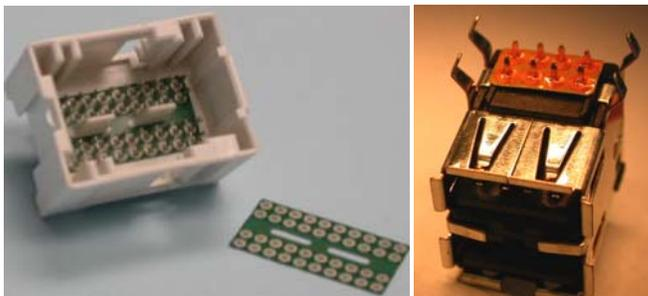
Figure 2. ESD Connector Array on 40 pin MQS automotive engine control module connector.
