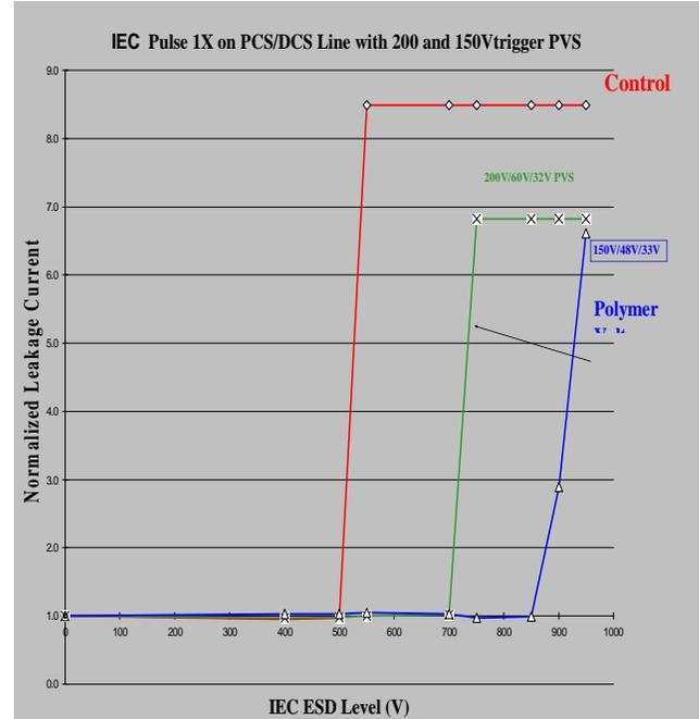
Figure 15: HBM testing of PCS/DCS module with 200V and 150V PVS device show ESD protection increases by 2x with 150V PVS device
