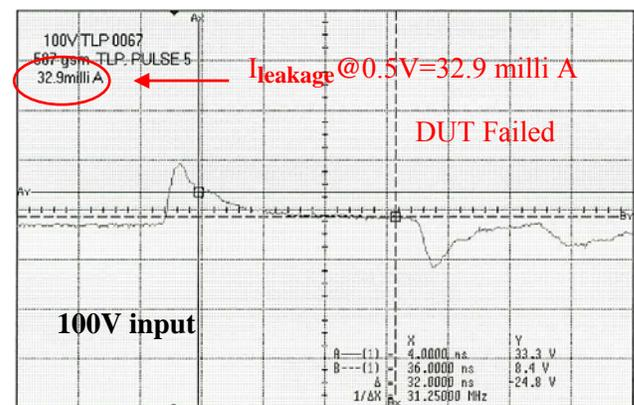
Figure 12: 100V TLP pulse into GaAs module increase damage to module
