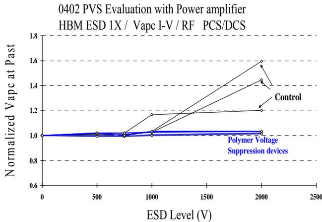
Figure 7: Device power setting degradation takes place at significantly lower ESD voltages without PVS protection.
