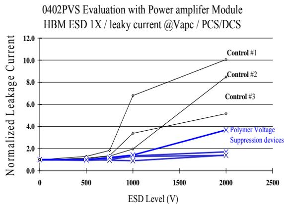
Figure 8: GaAs leakage degradation increases significantly at lower ESD voltages without PVS protection
