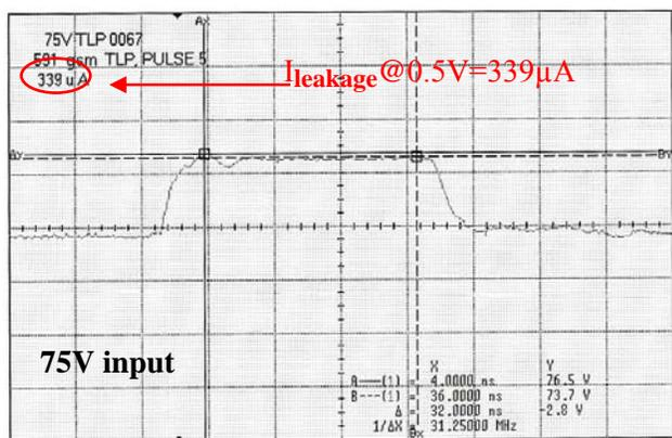
Figure 10: Scope trace for 75V TLP pulse into GaAs module shows no damage to the device
