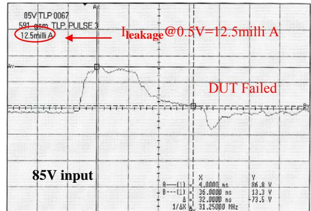
Figure 11: 85V TLP pulse in GaAs module damaged module
