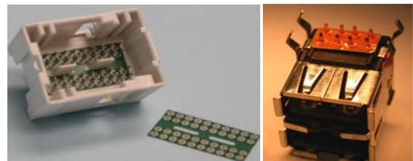
Figure 3: EPI-FLO™ ESD Connector Array on 40 pin MQS automotive engine control module connector and a RJ-45.
