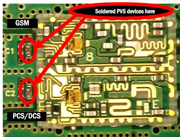
Figure 5: Dual GSM and PCS/DCS module site for soldering surface mount 0402 PVS ESD protection device
