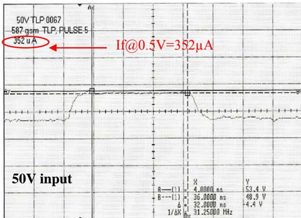
Figure 9: Scope trace for 50V TLP pulse into GaAs Module shows no damage to the device
