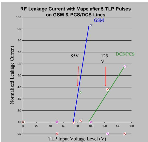
Figure 14: TLP damage threshold degradation curves from leakage current measurements at 1.5V
