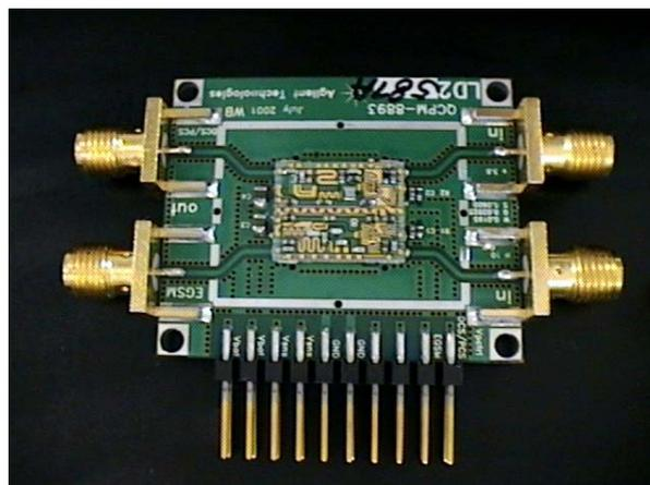
Figure 4: Demo board for Dual GSM and PCS/DCS module
