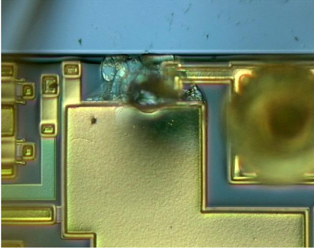
Figure 13: TLP Testing of GPS mode to failure shows visible damage on the device circuit
