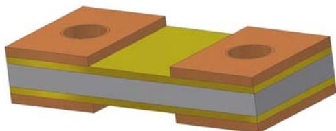
Figure 6: PVS Construction for 0603, 0402, 0201 Electronic Polymers Inc. EPI-FLO™
