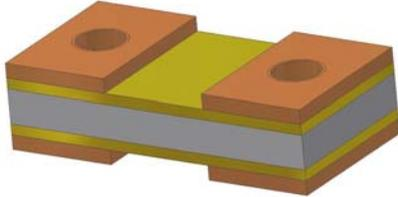
Figure 1: PVS Construction for 0603, 0402, 0201 Surface Mount Device
