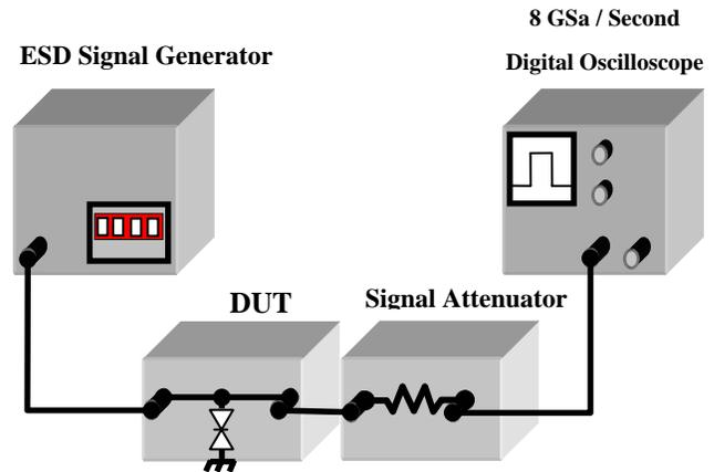
Figure 5: TLP set-up
