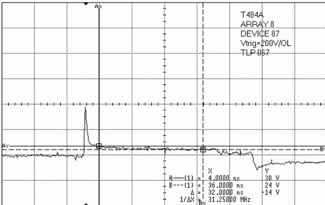
Figure 4: 200 V<sub>trigger</sub> 0603 PVS response to 200 V TLP.
