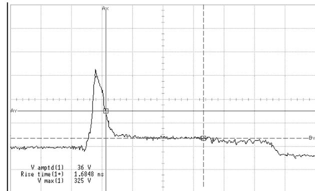
Figure 11: 600 V TLP into PVS protected RJ-45 Connector with magnetics on PCB in the connector
