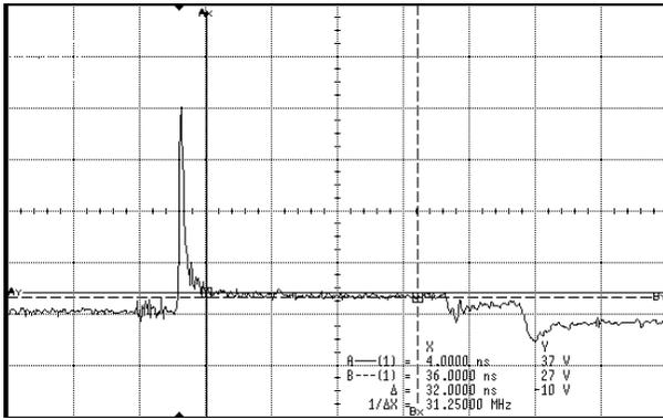
Figure 3: 0603 PVS device clamps 600 V TLP to 27 V
