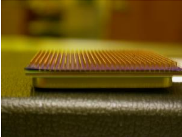
Figure 3: EPI-FLO™ connector array is made to be press fitted onto microprocessor chip.
