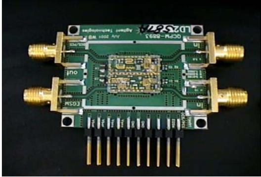
Figure 4: Demo board for Dual GSM and PCS/DCS module
